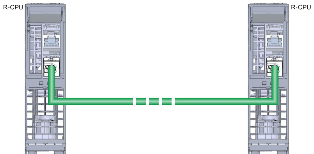
Figure 6-6 PROFINET interface X1 P2 R: Connecting R-CPU (bottom view)
